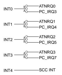
STEbus interrupts are level triggered, 188EB on-board peripherals can be configured to use edge- or level triggered interrupts.
