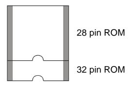
32 pin ROMs should take up the entire socket and should be fitted in the orientation shown in the 'Default Link Position' diagram.
